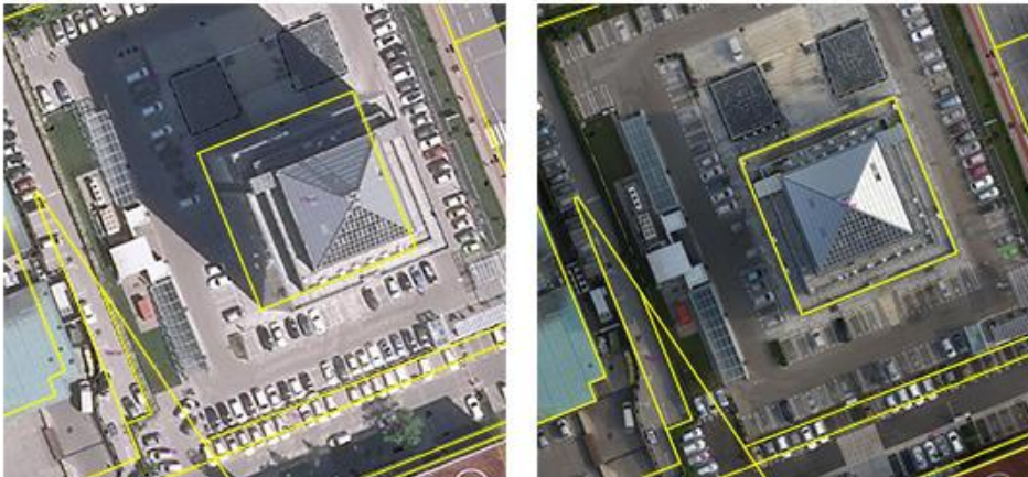
Comparison of a traditional (left) and true (right) orthophoto
